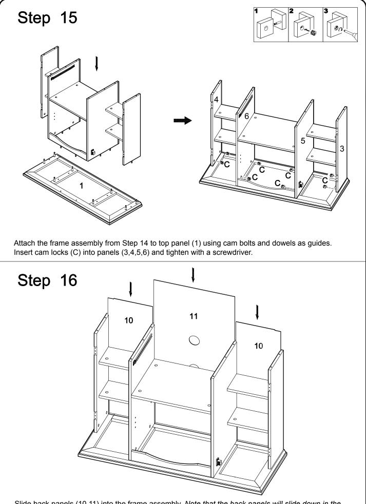
Slide back panels (10,11) into the frame assembly. Note that the back panels will slide down in the grooves along the back of the frame assembly.
